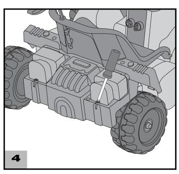
Replace the rear bumper cover (battery retainer) and tighten the screws.
